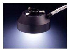
An indirect light. Illumination is reflected off the interior of the dome, resulting in  $360^{\circ}$  of even and diffuse illumination. Suitable for applications with high reflection and halo problems.
